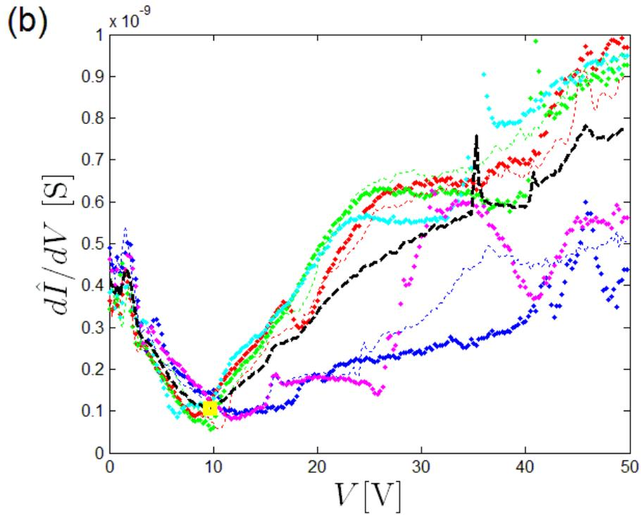
**FIG. S1. (Color online) (a) Individual I-V's per channel and (b) differential conductance per channel for Array F. The dashed black line marks the calculated mean while the large yellow square marks the point of the minimal average differential conductance and corresponding limiting current.**
