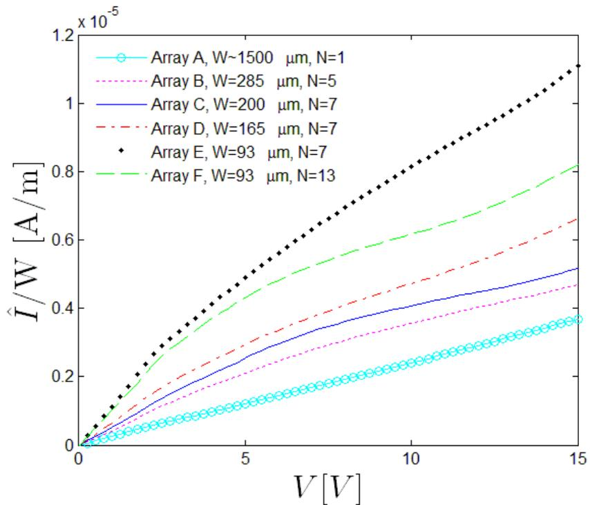
**FIG S2. (Color online) The current density per channel ,  $\hat{I}/W$  , for the various arrays. The predicted reversal [21,22] of the current density (per channel) compared to that of the current (per channel) behavior is confirmed.**
